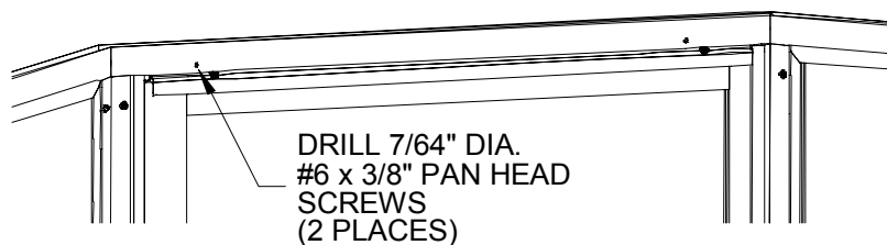
VIEW FROM INSIDE OF SHOWER
